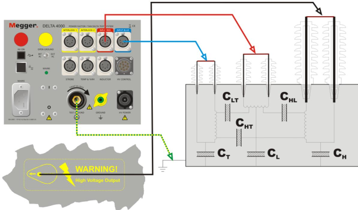
For CHT measurement UST-B should be selected. The blue terminal is now measured and the red is grounded. The time saving benefit is that the transformer can be tested without the need for reconnections.
