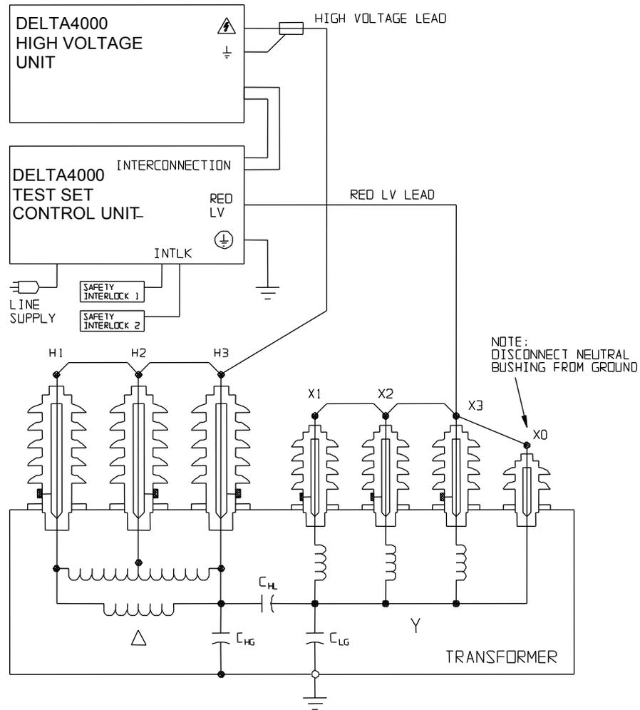
**Figure 4** Typical Test Setup for AC Insulation Testing of a Three-Phase Two-Winding Power Transformer
