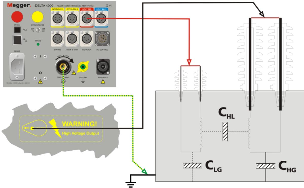
When UST-R is used for the CHL test, the HV output terminal is to be connected to the primary winding and the red terminal to the secondary winding. The blue terminal does not have to be connected in this case.
