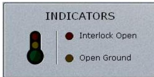
The indicators show if there are anything that prevents a measurement from starting. If the Interlock Open led is on, you have to close both switches before you can start a test.
