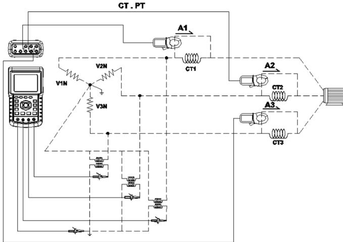
1. Power the instrument ON by pressing the 'Power' key (item 3-7; Section 3 diagrams), and then press the '1 $\Phi$  3 $\Phi$ ' key (item 3-22) to select the 3 $\Phi$  4W system, the selected name of the system will appear on the bottom left hand side of the display.
