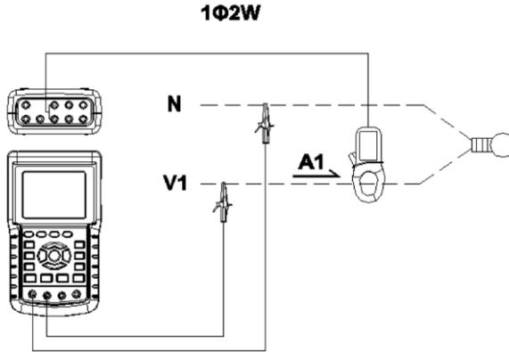
1. Power the instrument ON by pressing the 'Power' key (item 3-7; Section 3 diagrams), and then use the '1 $\Phi$  3 $\Phi$ ' key (item 3-22) to select the 1 $\Phi$  2W system, the selected name of the system will be shown on the bottom left side of the display (refer to Figure 5-1 below)
