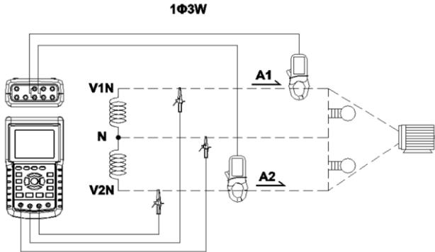
1. Power the instrument ON by pressing 'Power' key (item 3-7; Section 3 diagrams), and then press the '1Φ 3Φ' key (item 3-22) to select 1Φ 3W, the selected name of the configuration will appear on bottom left hand side of the display.
