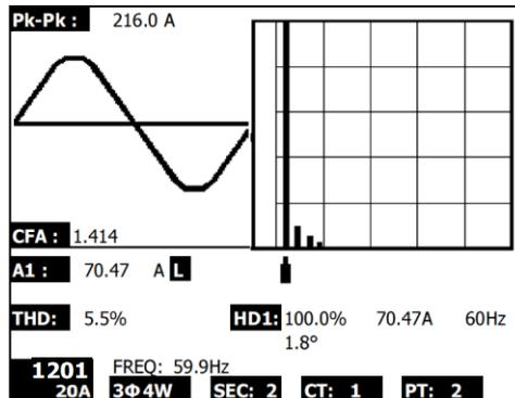
NOTE: If the waveform is clipped at the peak or too small in the LCD, press the RANGE button to select HIGH or LOW range for a better display. The range indicator is the symbol after the unit of RMS value, L or H.
