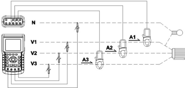
1. Power the instrument ON by pressing the 'Power' key (item 3-7; Section 3 diagrams), and then press '1 Φ 3Φ' (item 3-22) to select the 3Φ 4W system, the selected name of the system will appear on the bottom left hand side of the display.
