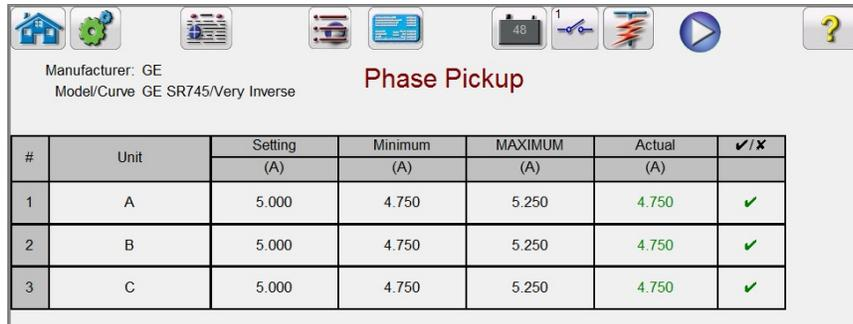
Figure 122 Example Phase Pickup and Dropout Test Screen
