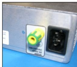
Figure 310 SMRT1 Rack Mount Back Panel Power Input
