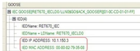
Figure 283 IED IP Address in the SCL File
