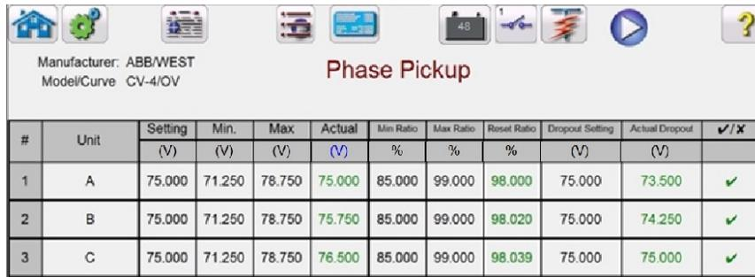
Figure 143 Example Phase Pickup and Dropout Test Screen
