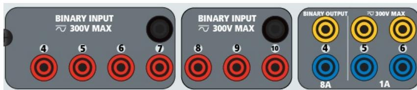
Figure 353 Binary Inputs 4 to 10 and Binary Outputs 4 to 6
