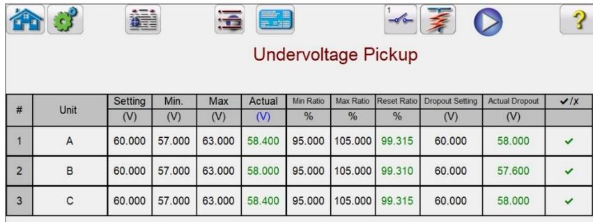
Figure 154 Example UV Phase Pickup Test Screen
