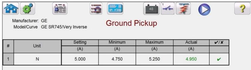
Figure 128 Example Ground Pickup Test
