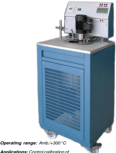
**Applications:** Control calibration of temperature sensors in laboratory, in conformity with ISO 9000 standards; Control of thermostats:
