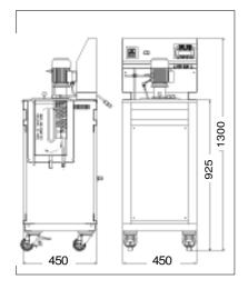
The TB300M bath is an instrument used to calibrate transducers, RTD and temperature-measuring sensors in the field and in the laboratory. The possibility to generate positive and negative temperature ramps makes it suitable for use in calibrating and testing thermostats.
