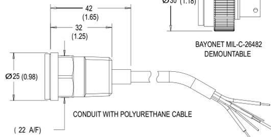
CONDUIT WITH POLYURETHANE CABLE
