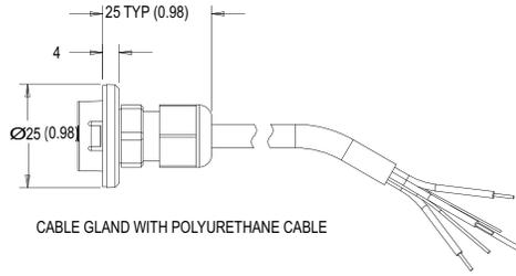
CABLE GLAND WITH POLYURETHANE CABLE
