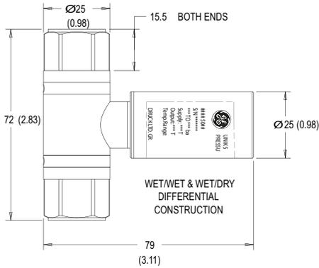
WET/WET & WET/DRY DIFFERENTIAL CONSTRUCTION
