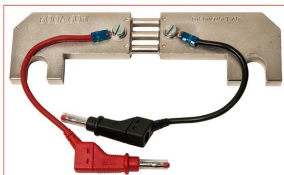
Calibration shunt MJÖLNER 600. Shunt 600 A/60 mV
