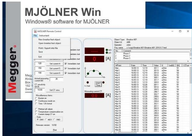
The MJÖLNER Win program makes it easy to manage/ save all test results in a simple way. All information, meta-data of the test object e.g. a circuit breaker and the test results are stored together and they can easily be transferred to Microsoft® Excel for further analysis. In MJÖLNER Win you can also save test files and print out test reports.
