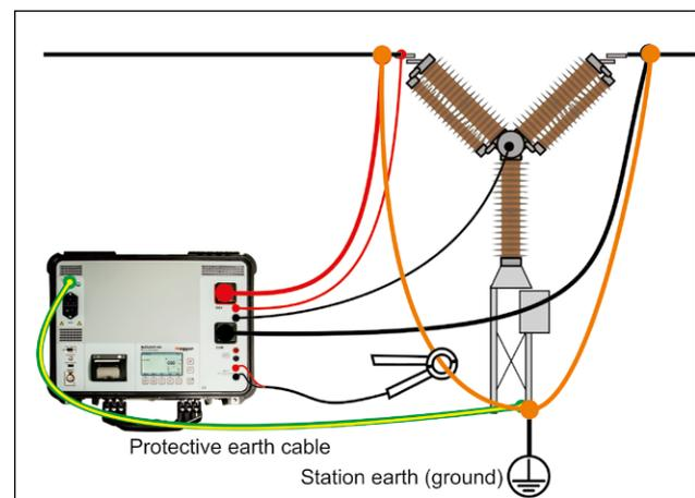
You can make tests with both sides of the test object grounded, an additional safety feature.
