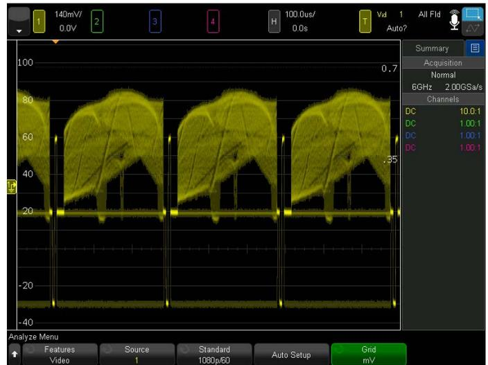
Figure 45. Triggering on a 1080p/60 signal.
