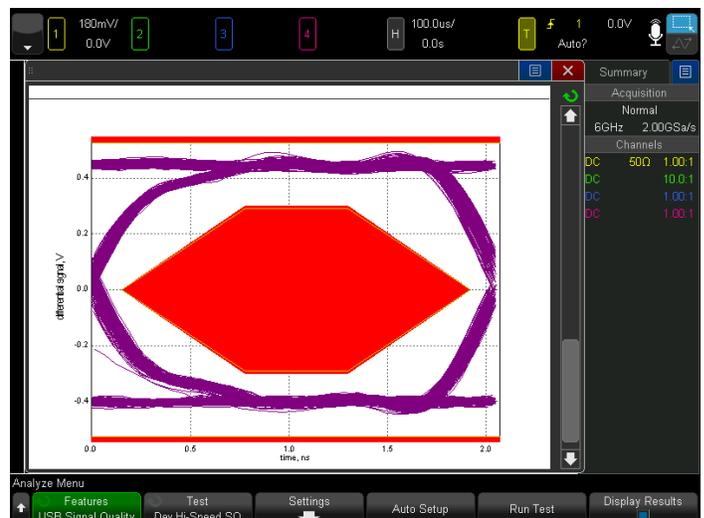
Figure 44. USB 2.0 Hi-speed near-end eye pattern test.
