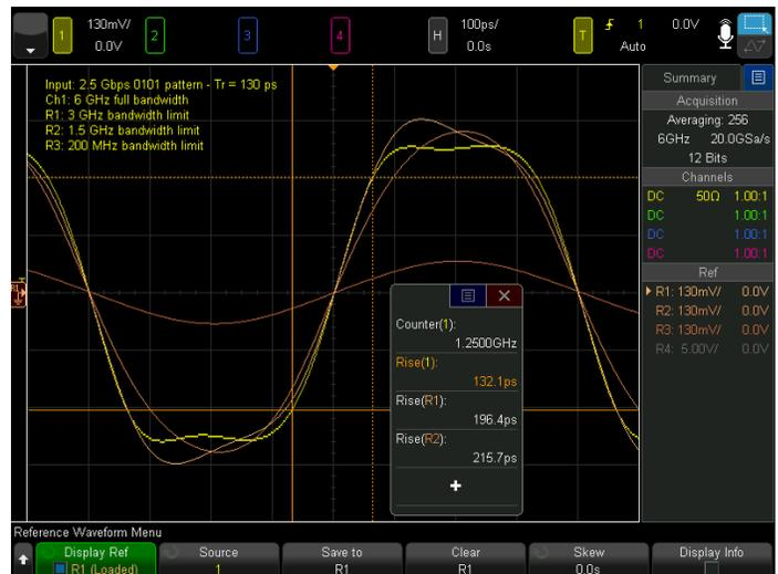
Figure 51. Reference waveforms.
