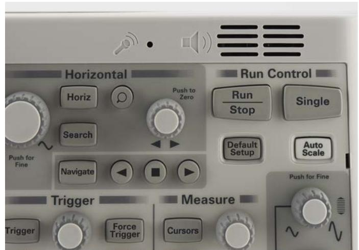
Figure 39. Voice control microphone and speaker.
