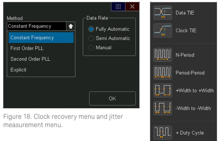
Figure 18. Clock recovery menu and jitter measurement menu.
