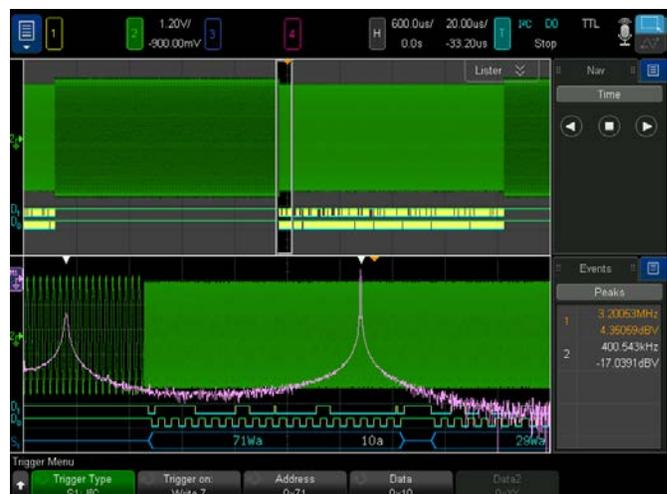
Figure 37b. Gated FFT time correlating the FSK frequency hopping with an I<sup>2</sup>C command (write 7 @ 0x71 data 10).
