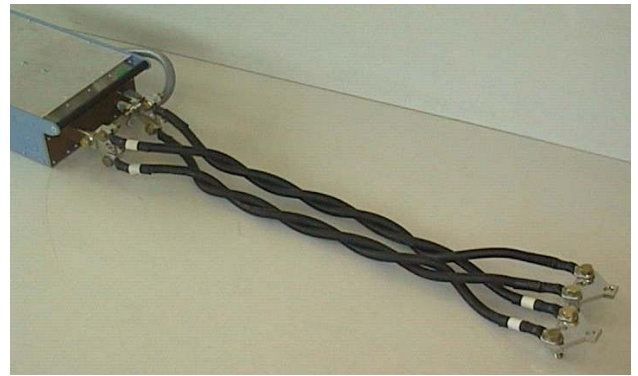
Current unit with twisted 2 pairs Multi-cable Set
