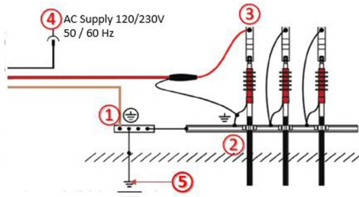
Resistance between grounding point of power device ① / ② and system earth and earth ground ⑤ **must be  $\leq 5\Omega$**
