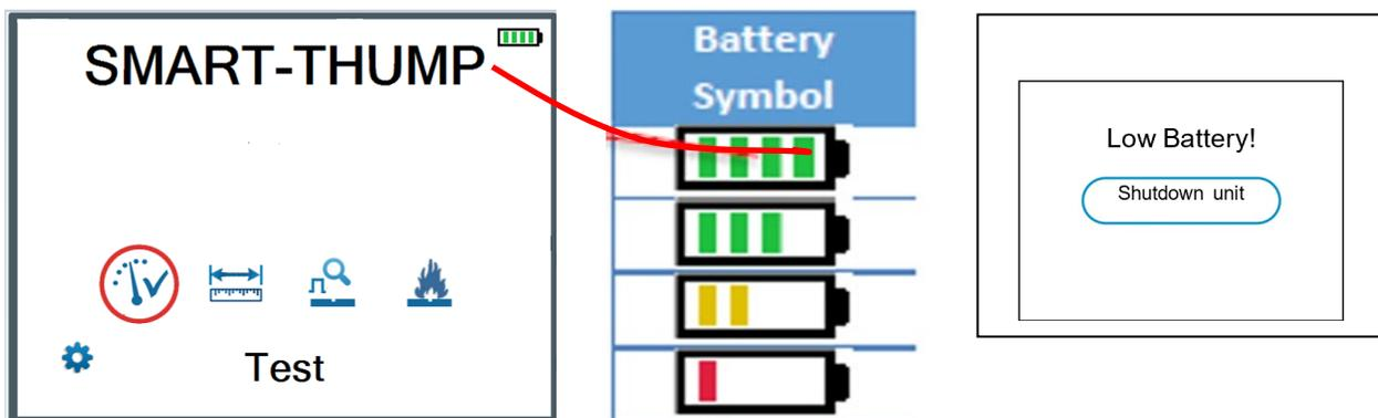
**NOTE:** *To protect the battery from a deep discharge, the unit turns off automatically completely or provides an error message if the battery is discharged too low for safe operation, see above.*
