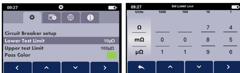
**NOTE :** The upper limit cannot surpass 3Ω and the lower limit can't surpass upper limit.
