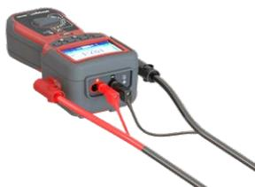
Once you have connected to the test object wait for "C" and "P" indicators to turn green, confirming proper continuity.
