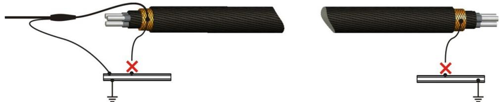
The insulation of any high or medium voltage shielded power cable is protected from water ingress by a jacket made from XLPE or PVC. The Sheath test checks *if* the integrity of the jacket has been compromised, typically during installation.
