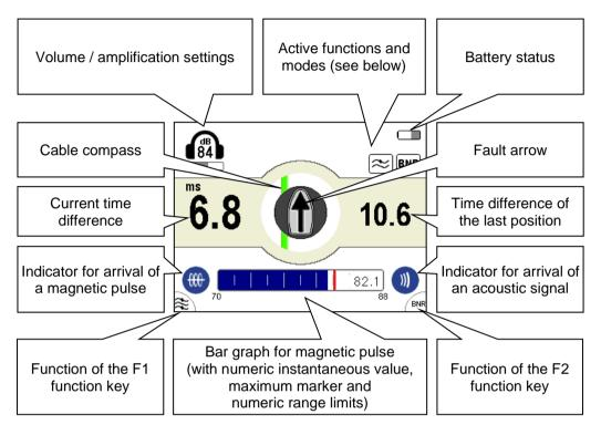
Active functions and The symbols at the top right of the measurement screen indicate the following functions modes and measurement modes:
