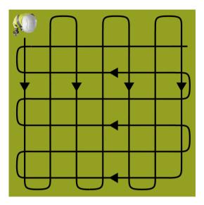
The sensitivity must be set to maximum at the beginning of the terrain examination. It is automatically reduced as soon as a signal response is detected. Each detected line should be routed and marked in both directions as far as the location at which it leaves the area that is being examined. Terrain examination should then continue.
