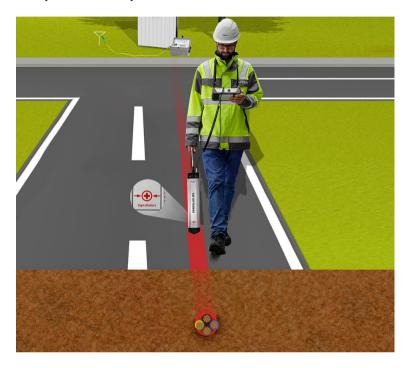
To ensure that the user has the most ergonomic posture possible, the handle of the receiver can be rotated around its axis in steps of 90°. To do this, push the handle downwards a little until it noticeably engages in the required position.
