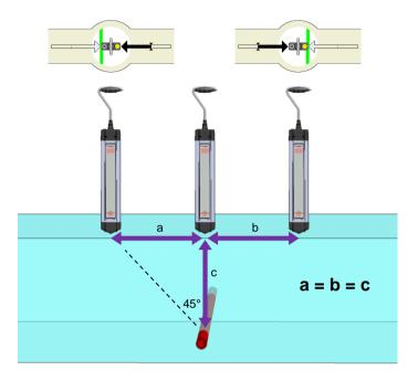
The situation is different if the transmitter signal is coupled into an adjacent line or a second supply line with the same mains frequency is running directly parallel to the line. A significantly less homogeneous field therefore forms around the lines, which leads to a significant difference between the measured distances.
