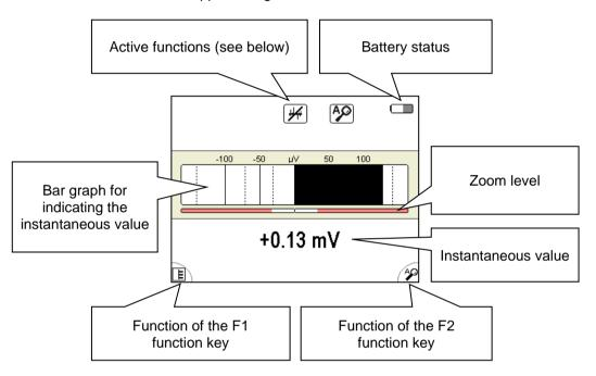
Active functions and The symbols at the top right of the measurement screen indicate the following functions modes and measurement modes:
