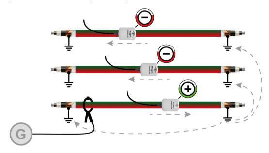
If it is not possible to couple the signals using a clamp, it is recommended to connect the transmitter directly to the cable shield. For this method, the cable shield must not be earthed on the connection side.
