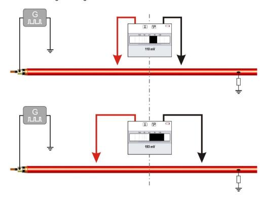
Particularly when you start pinpointing, it is advisable to place the earth spikes at larger distances from each other so that the generator impulse can be identified as clearly as possible, even at greater distances to the fault location.
