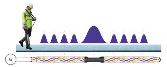
If the sleeve is very small, if the twist is continued inside the sleeve or if the cable is routed deeply, this method is not suitable for reliable positioning.
