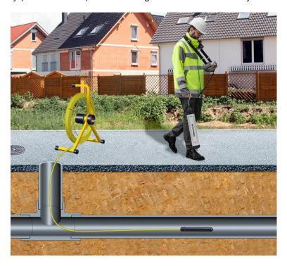
If the receiver is positioned directly above the probe and the two are aligned, the maximum signal is measured.
