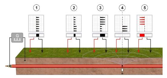
As voltage gradients induced by the current flowing back from the fault position exist around the earthing point of the generator, the measurement values near this point might be elevated (position 1). However, the deflection direction (polarity) also indicates the direction of the fault position at this point.
