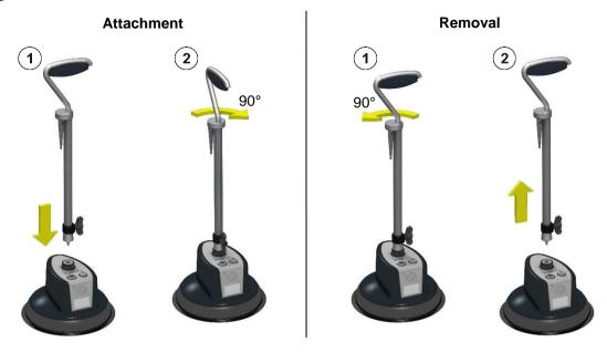
Adjusting the height of This is how to adjust the height of the telescopic handle: the telescopic handle
