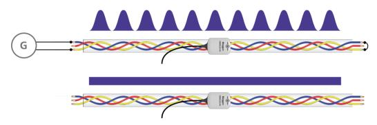
A consistent change in signal level will be measured from the inductively coupled cable, whereas the signal response from the neighbouring lines will remain relatively constant.
