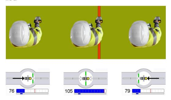
The filling of the arrow should decrease while approaching in the indicated direction, the signal level should increase and the green line should move further toward the centre. At the point of the absolute signal maximum (with minimum method: signal minimum), the receiver is located directly above the line.
