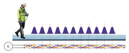
To perform this measurement, the audio frequency signal must be applied to a shortcircuited pair of wires and the highest possible current must be set at the generator. For twist measurements, the depth at which the cable is routed should not be greater than the length of a twist.
