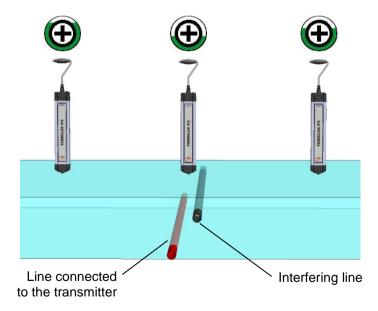
This is due to the fact that the influence of the weaker, overcoupled signal decreases as the lateral distance increases, and the actual signal on the line on which it is being transmitted can be clearly determined again accordingly.
