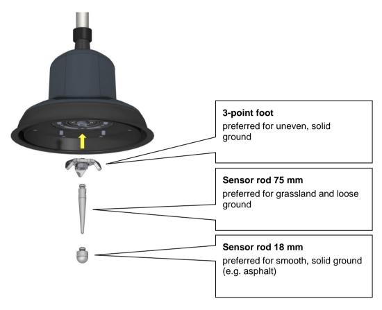
The 18 mm rod and the 3-point foot can both be used on smooth and solid ground. Because their acoustic qualities are different, it is for the operator to decide which probe they prefer to use on such ground.
