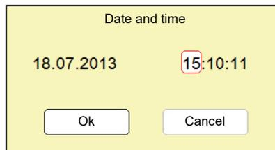
By tilting the rotary encoder **6** to the side the user can switch back and forth between the individual buttons in a dialog box. Each active button is then highlighted in white or it is surrounded by a red frame. Whenever the selected button requires letters or digits to be entered the screen keyboard automatically appears, and it can then be used to make the entries.
