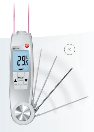
The testo 104-IR is a waterproof (IP65) penetration thermometer combined with an infrared sensor for non-contact temperature measurement. It can be used for all sorts of applications in the food sector. The testo 104-IR scans the surface temperature of individual foods or entire goods pallets without contact, particularly in the Incoming Goods department. If a limit value is exceeded or undershot, the hinged penetration probe is also able to measure the core temperature.
