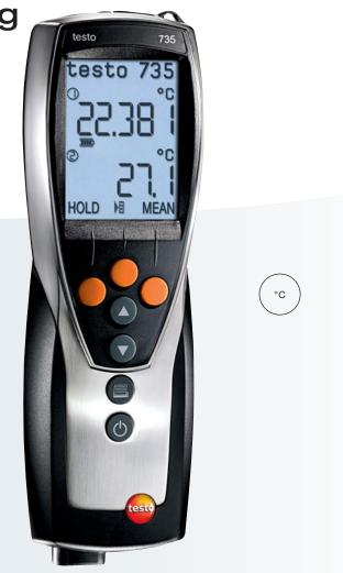
The robust and compact measuring instrument testo 735 is universally applicable and is available in two versions: testo 735-1: Precise temperature measuring instrument without measurement value store
