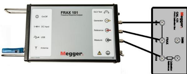
Measure from 10 Hz to 10 MHz and the measured data should be 0 dB with a maximum deviation of +/-0.1 dB.
