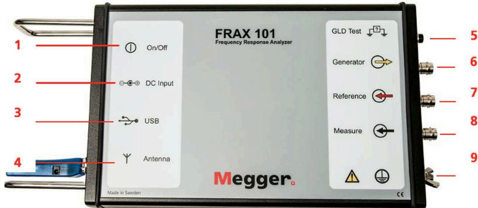
1. **On / Off** To turn the instrument on/off
