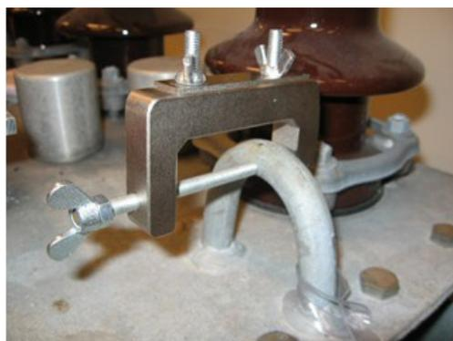
The G-clamp is easy to attach, easy to tighten the braid, which ensuring a quick and reliable procedure for shortest braid practice, which is essential to get repeatable measurements.
